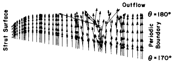
FIG. 15. Velocity on midspan plane ( z = 0.0 ) preceding outflow boundary indicating solution breakdown due to insufficient spatial resolution (elliptical strut with Re = 1000 ).
